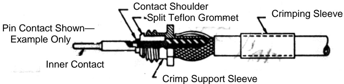
**Step 6)** Insert the terminated inner contact assembly into the threaded end of the contact outer body and tighten the outer body to the crimp support sleeve to 6 inch pounds maximum using a 13/64 open end wrench to hold the support sleeve
